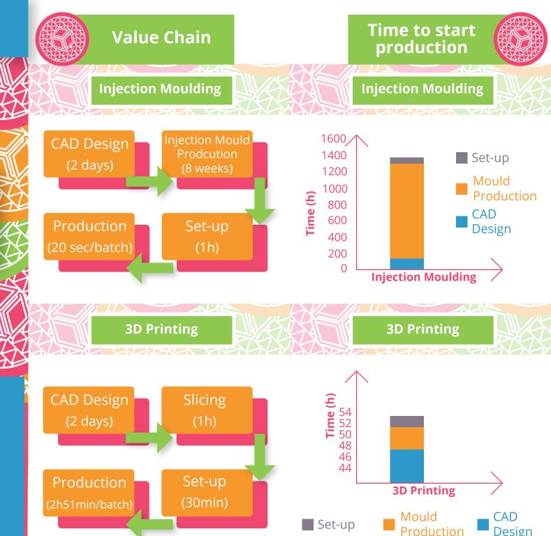
The following flyer showcases a small case study based on the AMable coin made for the purpose of this event. A comparison between 3D Printing and injection moulding is made. Nevertheless, it is important to highlight that the aim of this document is not to prove that one is better than the other, but to showcase that these technologies are used in different applications, depending on the volume of parts produced and the variation of properties.
