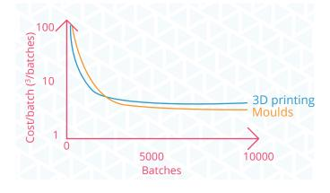
In terms of production costs, 3D printing is more advantageous up 4958 sets, being the cost per set of around 4.5€. As expected, the higher investment with the injection mould would require more batches to be cost effective.
